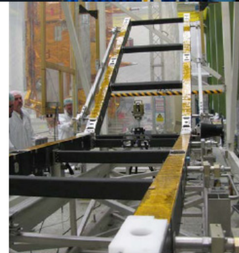
SAR Antenna Panel A during Antenna Pattern Tests and SAR Antenna Panel Frames D and E during integration of Deployment Mechanisms (Courtesy of Astrium GmbH, D)
