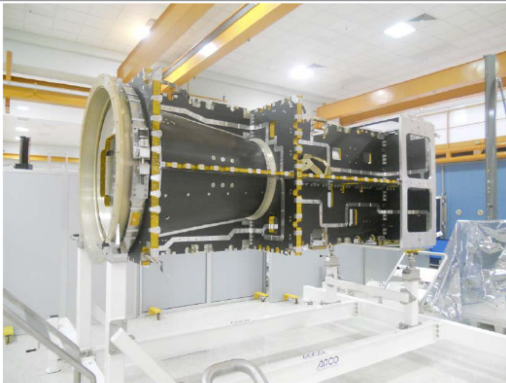
S/C Structure without external panels (Courtesy of TAS-I, I)
